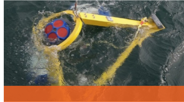
Figure 1: Acoustic Doppler Current Profiler (ADCP)
